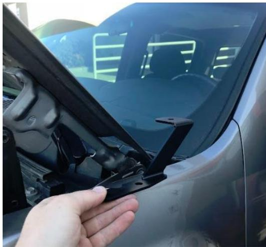
5. The bracket can now be moved into position carefully as to not scratch the body of the vehicle.
